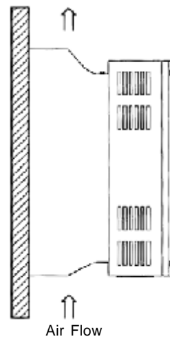
Figure 8.27 - DBW-01 and DBW-02 Positioning
