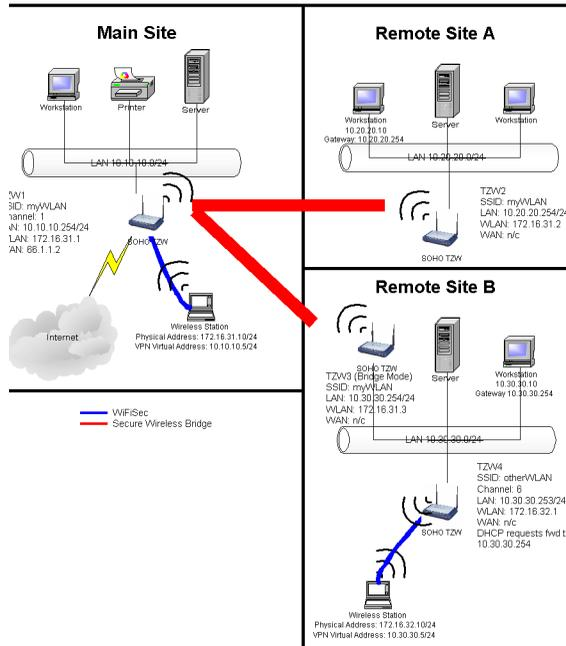
Secure Wireless Bridging employs a WiFiSec VPN policy, providing security to all communications between the wireless networks. Previous bridging solutions offered no encryption, or at best, WEP encryption.
