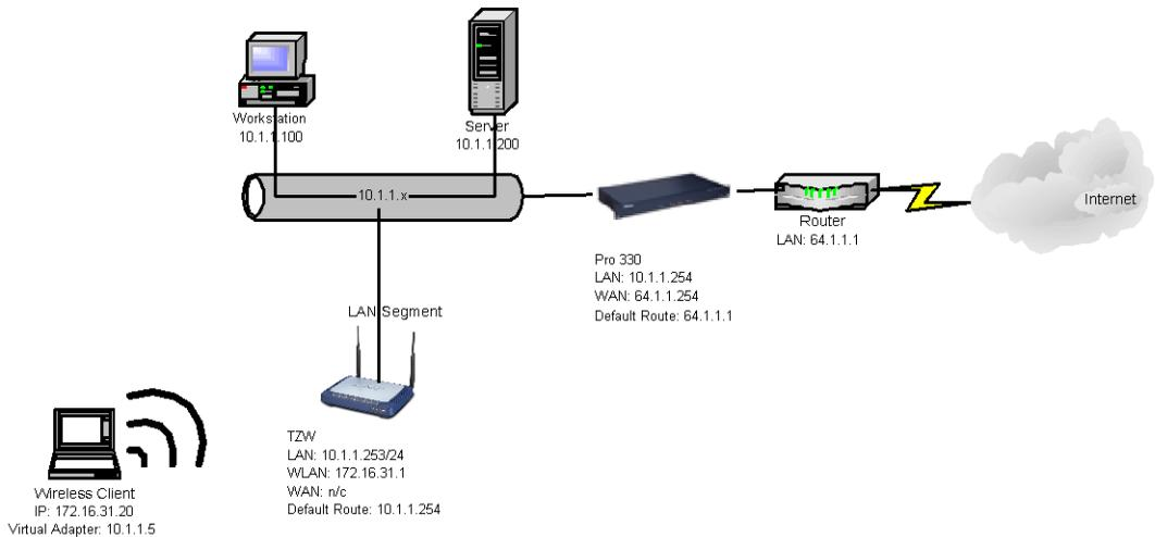
The above example shows a network configuration with the addition of a SOHO TZW (as a Secure Access Point). The SOHO TZW points to the upstream SonicWALL PRO 330 at 10.1.1.254. Security Services, such as Content Filtering Service and Anti-Virus, are hosted centrally on the PRO 330. In the example above, PRO 330 does not require a route to the 172.16.31.X as long as the Virtual Adapter is used by all clients.
