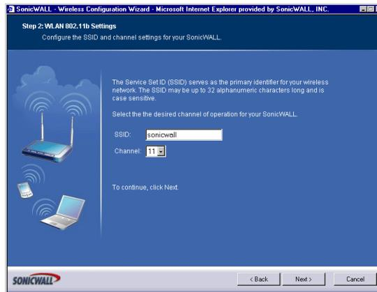
3. Type a unique identifier for the SOHO TZW in the SSID field. It can be up to 32 alphanumeric characters in length and is case-sensitive. The default value is **sonicwall**.
