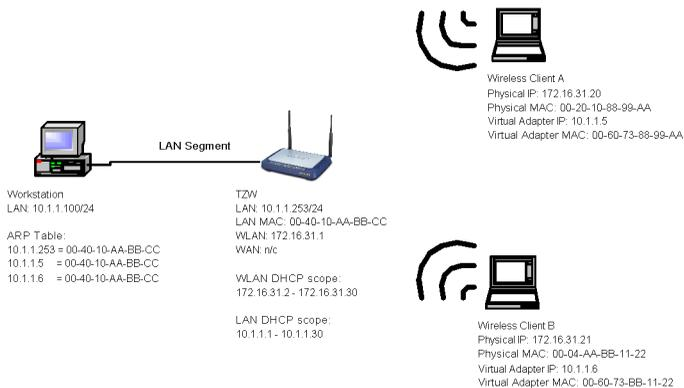
This allows any client on the LAN to communicate directly with WLAN client via the secure WiFiSec link, enabling configurations like the one below.
