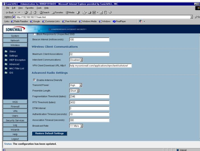
Clearing the **Enable Antenna Diversity** checkbox presents a pop-up message indicating that only the antenna nearest the power-socket is active when antenna diversity is disabled. The antenna nearest the serial connector **must be disconnected** when antenna diversity is disabled. The optional antenna should then be connected to the RP-TNC type connector near the power-socket. This antenna is not used exclusively for transmitting and receiving.
