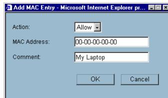
2. Select **Allow** from the **Action** menu to allow access to the WLAN. To deny access, select Block.
