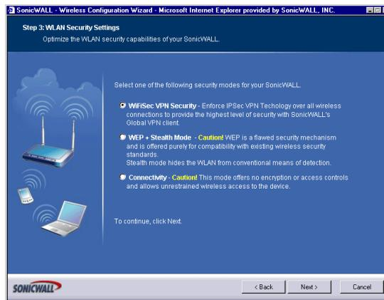
4. Choose the desired security setting for the SOHO3 TZW. **WiFiSec** is the most secure and enforces IPsec over the wireless network. If you have an existing wireless network and want to use the SOHO TZW, select **WEP + Stealth Mode**.
