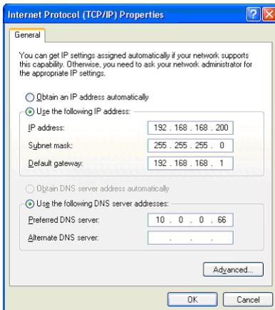
3. Select **Use the following IP address** and type **192.168.168.200** in the **IP address** field.
