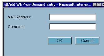
5. In the **Add WEP-on-Demand Entry** window, enter the MAC address of the wireless device in the **MAC Address** field.
