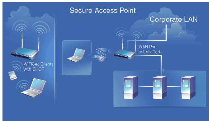
Any LAN clients attempting to resolve an IP address of a Global VPN Virtual Adapter address receives a response from the SOHO TZW LAN.
