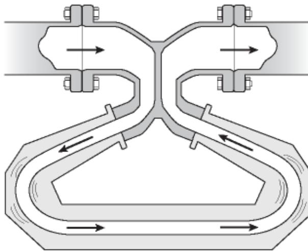
**Figure 4: Coriolis Flowmeter**
