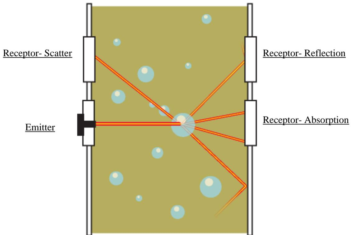
**Figure 3: Signal Receptors for Spectroscopic Water Cut Device**
