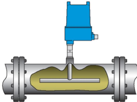
**Figure 6: Spool-Piece Cut Monitor**
