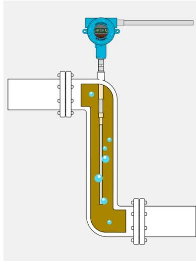
**Figure 7: Pipe Insertion Cut Monitor**
