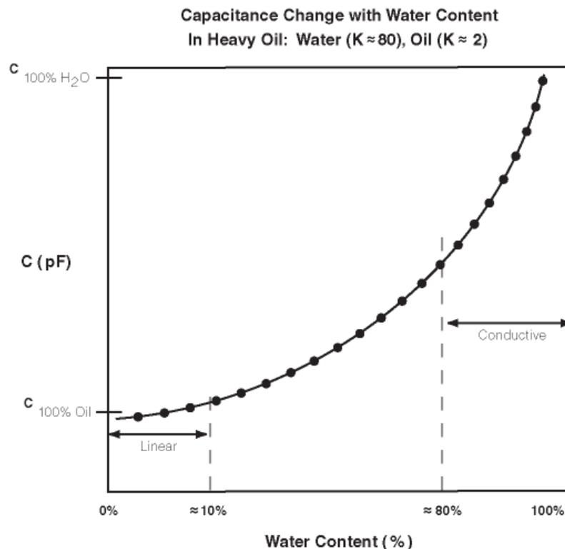
**Figure 2: Correlation of Capacitance to Water Content**
