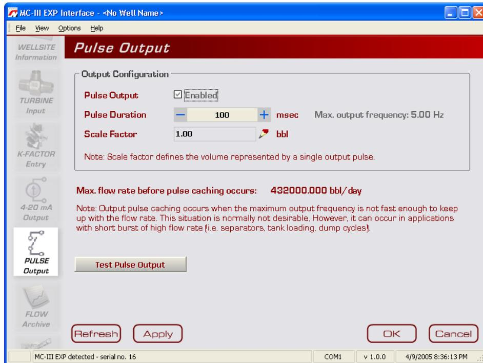
Figure 4.32—Pulse Output screen
