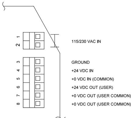
Figure 3. Power Connections
