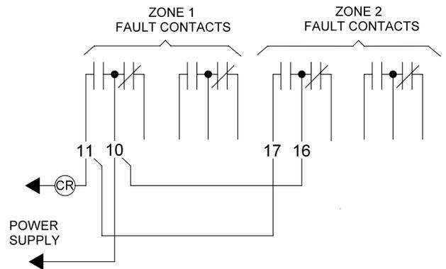
Figure 11. To Energize External Load (relay coil, etc.)
