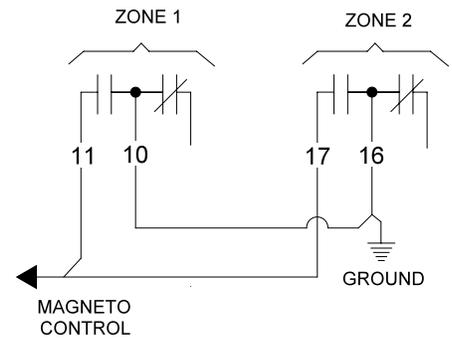
Figure 9. Magneto Grounding
