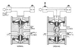
**NORMAL** Design employs principle of imbalance wherein the supply pressure is applied to the greater effective area on the bottom side of the lower diaphragm.
