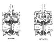
**NORMAL** Design employs principle of imbalance wherein the supply pressure is applied to the greater effective area on the bottom side of the lower diaphragm. Pressure is also fed to the top diaphragm through an orifice in the stem and is vented through bleed orifice.
