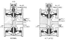
**NORMAL** Design employs principle of imbalance wherein the supply pressure is applied to the greater effective area on the bottom side of the top diaphragm.
