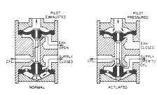
**NORMAL** Design employs principle of imbalance wherein the supply pressure is applied to the greater effective area on the bottom side of the lower diaphragm.
