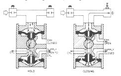
**HOLD** In the "Hold" actuated position, the internal compensating orifice compensates for minor leaks present in the pilot system.
