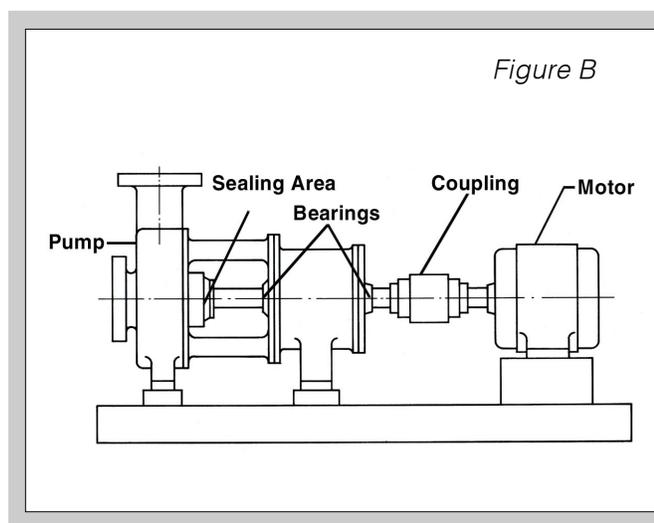
Dynamic seals are frequently located on the shaft of a centrifugal pump. The pump converts the electric motor's rotating energy into velocity, or pressure energy of the liquid or gas being moved.
