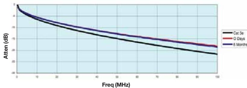
A six-month long test, fully submerged in water: top chart depicts the extensive attenuation degradation of the COTS cable; the bottom chart shows the superior performance of Belden DataTuff 7934A.
