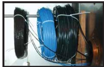
**The cables were tested, as suspended, in a high temp oven.**
