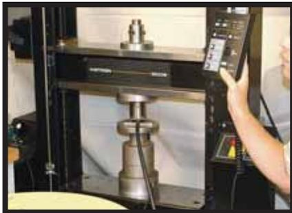
The Instron crushing device.
