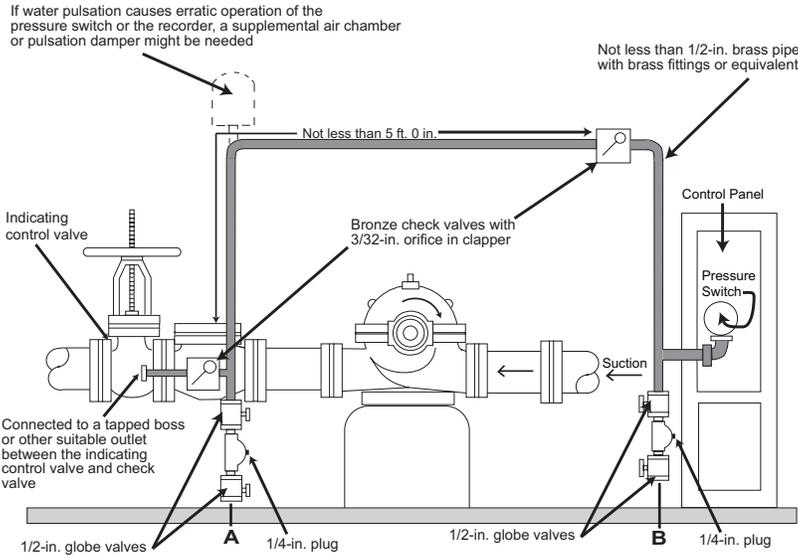
**Figure A.10.5.2.1(a) Piping Connection for Each Automatic Pressure Switch (for Electric Fire Pump and Jockey Pumps).**
