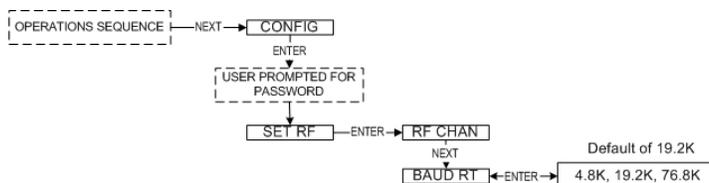
Figure 5.2: Menu Map to Baud Rate Setting
