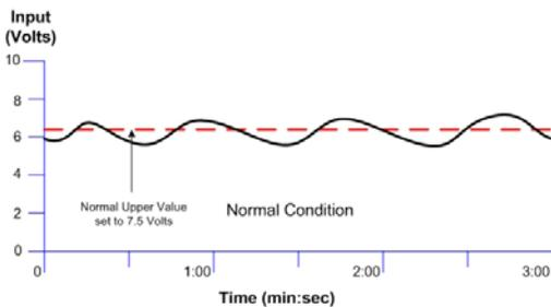
Figure 6.12: Condition "Chatter" Elimination Due to Time Deadband
