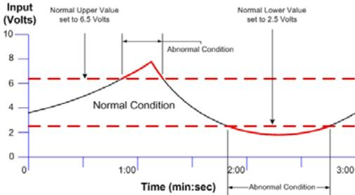
Figure 6.9: Normal Upper and Lower Value Example
