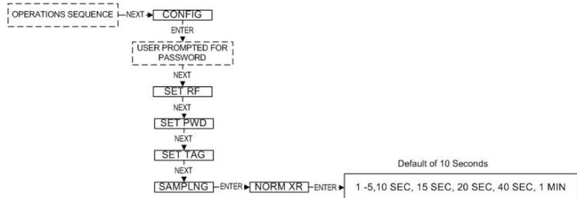
Figure 6.1: Menu Map to Normal Transmission Rate Setting
