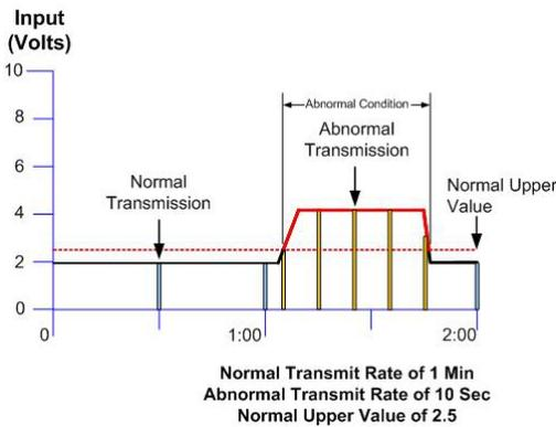
Figure 6.5: Example of Abnormal Transmission Rate Setting
