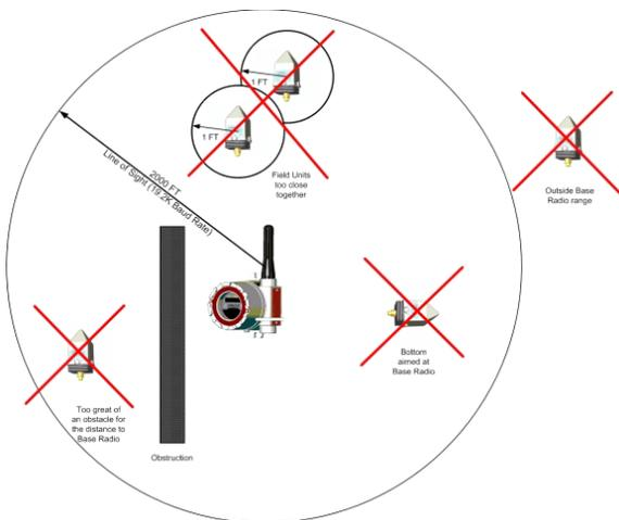
Figure 3.1: Examples of Incorrect Field Unit Positioning
