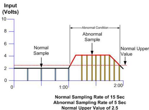
Figure 6.7: Example of Abnormal Sampling Rate Setting
