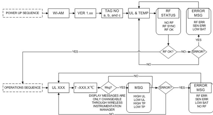
Figure 4.1: Field Unit Power-Up and Operations LCD Sequences
