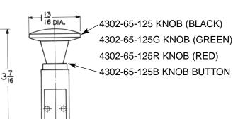
Large-diameter black plastic button is standard, for comfortable operation. Green Knob or Red Knob is available. See suffix options below. Nominal operating force is 3.75 lb. + .05 times line pressure.
