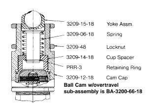
Can be operated by a cam or machine member. Has 3/16" overtravel after full actuation. This valve can be panel mounted. Pressure angle should not exceed 15° from vertical center line. Cam follower is hardened 430F stainless steel.
