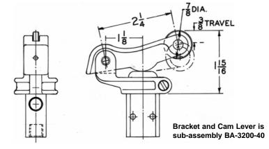
Actuated by cam movement in either direction. Cam follower is hardened.
