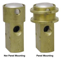
WITH GUARD: For fingertip or straight-line mechanical operation. Button is flush with extended guard to protect against accidental actuation. Aluminum button travels 3/16" for full actuation. Nominal operating force is 3.75 lb. + .05 times line pressure.
