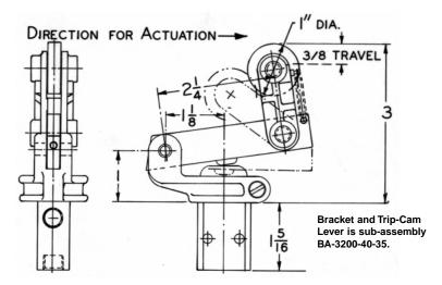
Actuated by cam travel in one direction only. Overriding device prevents actuation on return stroke. Cam follower is hardened.
