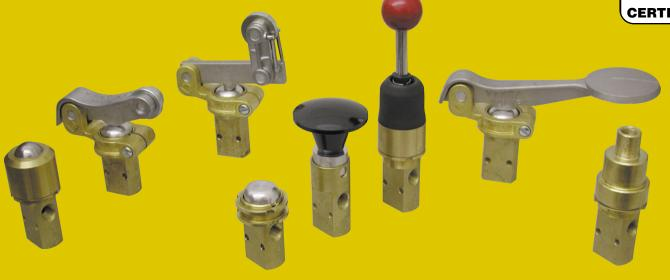
**Two-Way Types** for bleeding pilots of larger valves, for bleeding cylinders or small pressure systems, operating air tools or motors, opening or closing air lines. **Three-Way Types** for controlling pilots or diaphragms of larger valves or small cylinders...or any pressure system that is alternately pressurized and exhausted. **Service:** Pneumatic-vacuum to 200 psi (14 bar). Two-way can be used for hydraulic pressures to 500 psi.
