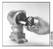
The transmitter electronics board is located in the compartment opposite the terminal side. To remove the electronics board perform the following procedure:
