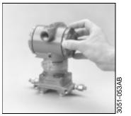
4. Replace the electronics housing cover. The transmitter covers must be engaged metal-to-metal to ensure a proper seal and to meet explosionproof requirements.
