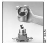
1. Carefully tuck the cable connector completely inside of the internal shroud.
