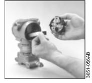
1. Remove the cable connector from its position inside of the internal shroud and attach it to the electronics board.
