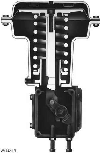
Figure 3-34. Diaphragm Actuator for Rotary Shaft Valves
