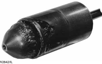
Figure 5-6. Typical Appearance of Flashing Damage
