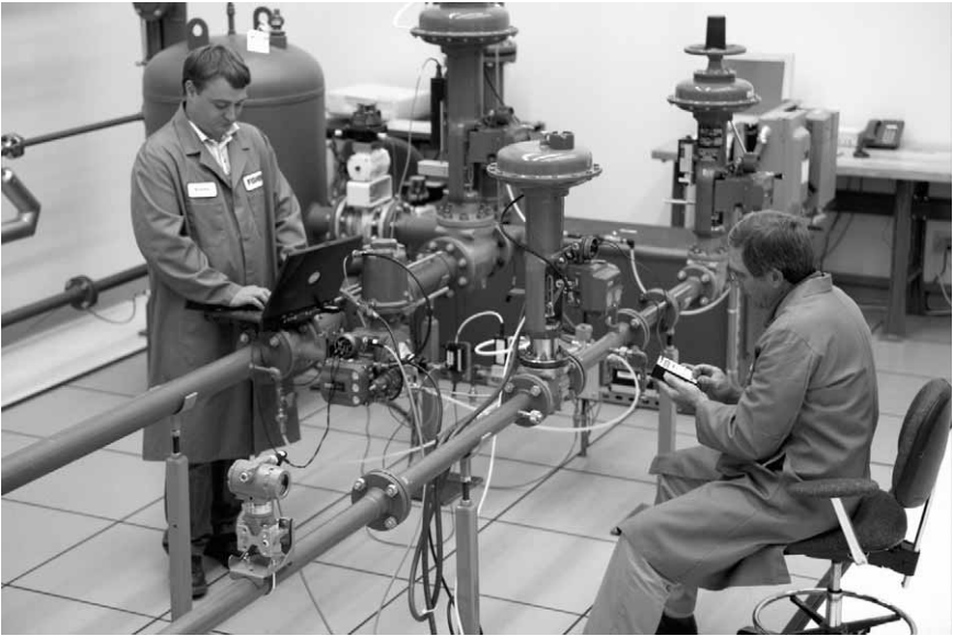
Figure 2-2. Performance Test Loop
