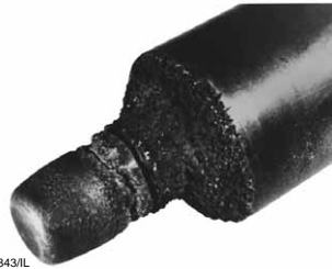
Figure 5-7. Typical Appearance of Cavitation Damage
