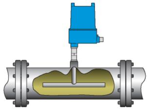
**Figure 6: Spool-Piece Cut Monitor**
