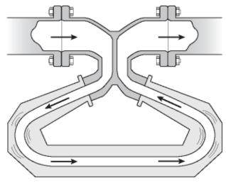
**Figure 4: Coriolis Flowmeter**
