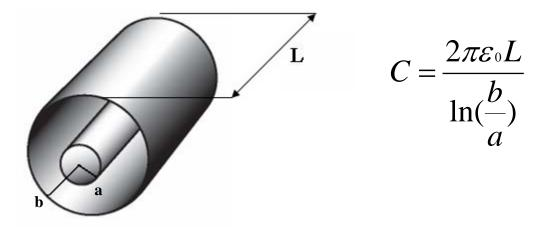
Figure 1: Standard Cylindrical Capacitor
