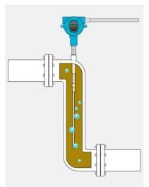
**Figure 7: Pipe Insertion Cut Monitor**
