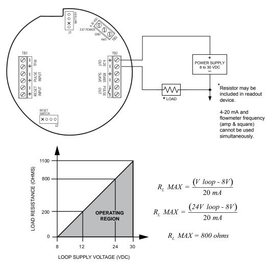
Figure 2.14—4-20 mA rate output wiring
