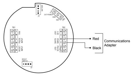
Figure A.6—Circuit board connection for communications adapter
