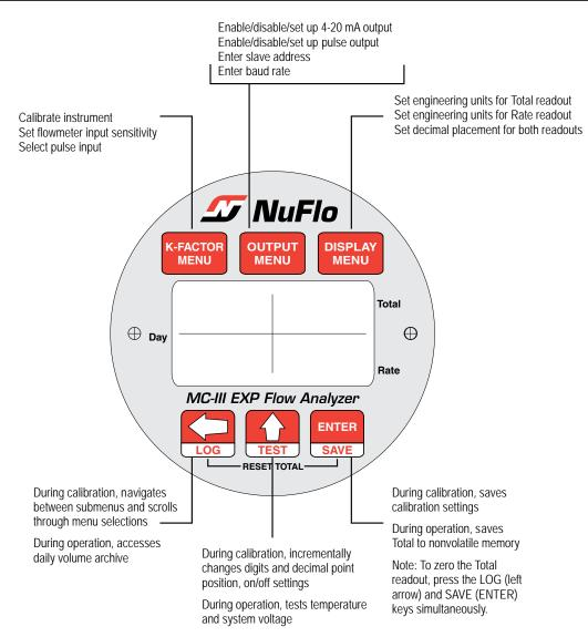
Figure 1.5—MC-III EXP keypad functions
