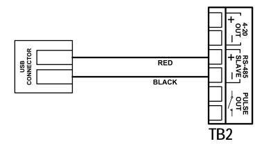
Figure A.10—Wiring of NuFlo USB adapter (required only when purchased as a kit)
