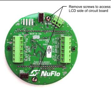
Figure 6.5—Disassembly of circuit board/keypad assembly
