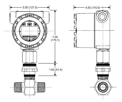
Figure 2.6—Direct mount (alternate MC-III EXP enclosure) to NuFlo turbine meter with pipe reducer and union (CSA)
