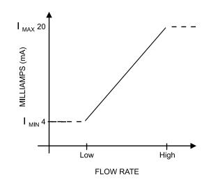
Figure 4.29—4-20 mA output configuration
