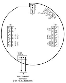
Figure A.2—Explosion-proof switch wiring
