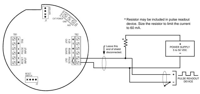
Figure 2.13—Pulse output wiring
