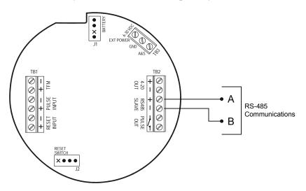
Figure 2.16—RS-485 output (permanent connection)
