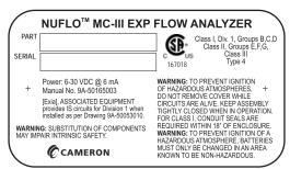
Figure 1.2—Serial tag for CSA-approved device
