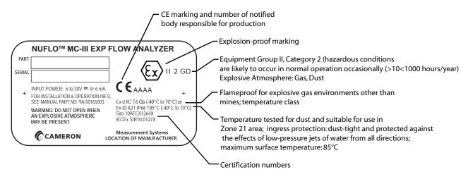
Figure 1.3—Serial tag for ATEX-approved device
