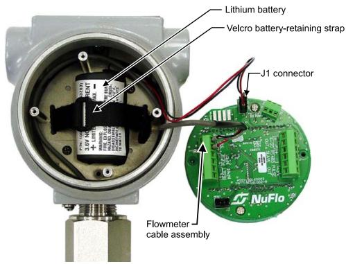
Figure 6.2— Removal/replacement of lithium battery
