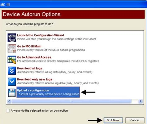
Figure 4.38—Upload a Configuration option
