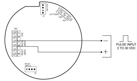
Figure 2.10—Pulse input wiring
