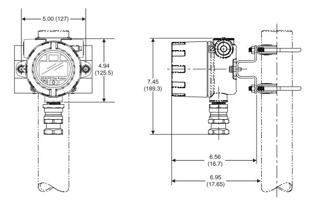
Figure 2.4—Remote mount on a 2-in. pole using a NuFlo hardware kit (Part No. 9A-30028004)
