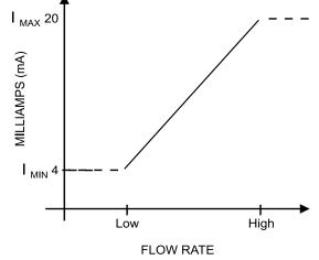
Figure 3.2—4-20 mA output configuration
