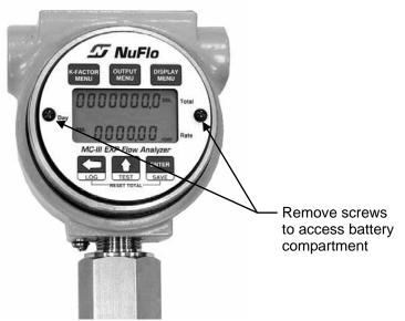
Figure 6.1— Removal of faceplate/keypad assembly
