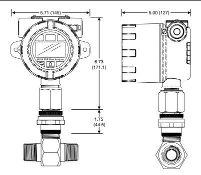
Figure 2.5—Direct mount (standard MC-III EXP enclosure) to NuFlo turbine meter with pipe reducer and union (CSA)
