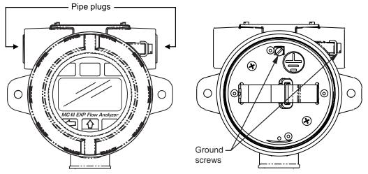
Figure 2.1—Enclosure entry and ground screw locations
