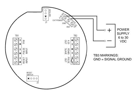
Figure 2.8—External power supply wiring
