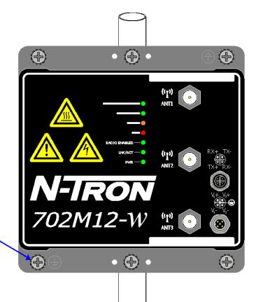
6x Tighten #10-32 screws until split lock washers fully compress (all installations)
