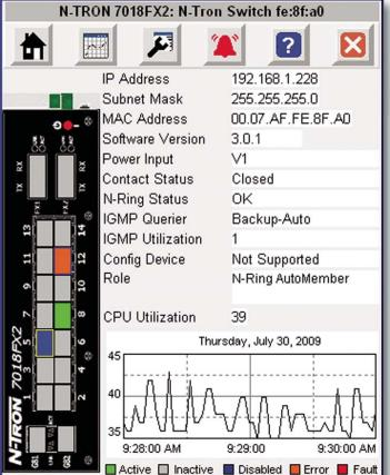
Quickly view switch status using our provide face plates or access tagged data from your ladder logic program.
