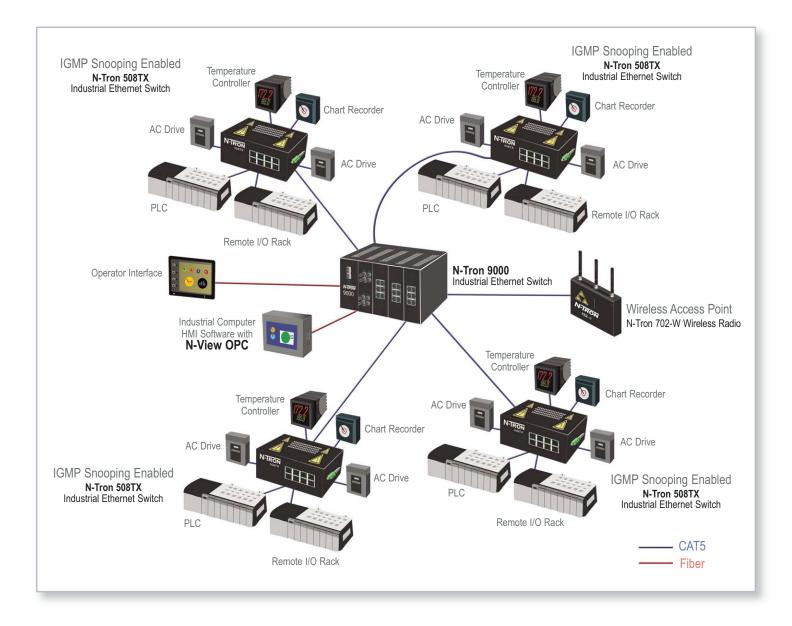
The tree topology uses a combination of several switches to form a single network. This topology provide the most efficient method of interconnecting multiple control systems. The above diagram highlights the Internet Group Management Protocol (IGMP). IGMP is frequently used by control systems to route multicast packets for communication between control devices.
