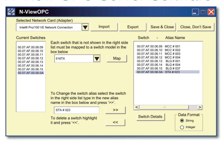
The N-Tron N-View<sup>™</sup> OLE for Process Control (OPC) Server Software will work with industry standard OPC Client software and most popular Human Machine Interface (HMI) packages, providing complete remote network traffic and status monitoring for N-Tron 300, 500, and 900 Series Industrial Switches with the N-View Firmware option. N-View is available as a standard feature on all 700, 7000, and 9000 Series Switches.
