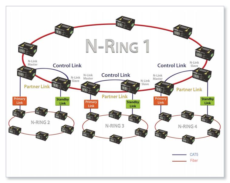
**The N-Link topology** allows the connection of two or more N-Rings to provide added hardware redundancy or to run interconnected N-Rings for a distributed N-Ring topology. The N-Link connections form redundant media links between two N-Rings and will monitor them to determine if the links are intact. If a break in the primary link occurs, traffic will be rerouted through the standby link within 30ms. A single N-Ring can support up to 126 N-Linked N-Rings.
