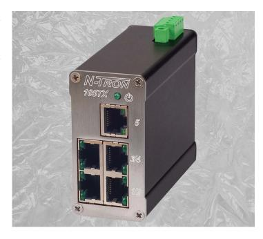
The 105TX supports up to 2,000 MAC addresses, enabling these products to support extremely sophisticated and complex network architectures.
