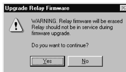
Figure 4–6: UPGRADE RELAY FIRMWARE WARNING
