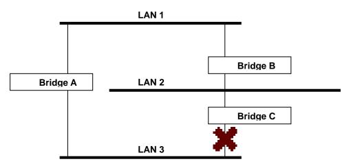
STP will determine which path between each bridged segment is most efficient, and then assigns a specific reference point on the network. When the most efficient path has been identified, the other paths are blocked. In the previous 3 figures, STP first determined that the path through Bridge C was the most efficient, and as a result, blocked the path through Bridge B. After the failure of Bridge C, STP re-evaluated the situation and opened the path through Bridge B.
