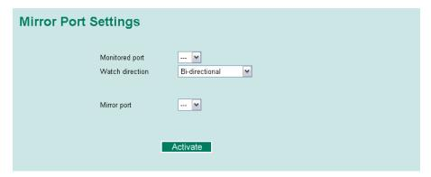
The **Mirror port** function can be used to monitor data being transmitted through a specific port. This is done by setting up another port (the *mirror port*) to receive the same data being transmitted from, or both to and from, the port under observation. This allows the network administrator to "sniff" the observed port and thus keep tabs on network activity.
