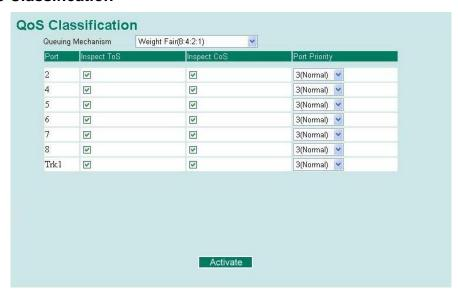
MOXA EDS-508A/505A supports inspection of layer 3 TOS and/or layer 2 CoS tag information to determine how to classify traffic packets.
