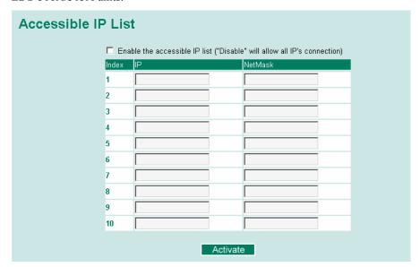
Accessible IP Settings allows you to add or remove "Legal" remote host IP addresses to prevent unauthorized access. Access to EDS-508A/505A is controlled by IP address. If a host's IP address is in the accessible IP table, then the host will be allowed access to the EDS-508A/505A. You can allow one of the following cases by setting this parameter:
