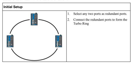
You do not need to set the Master to use Turbo Ring. Master is only needed to identify which segment acts as the backup path. The actual topology of the redundant ring, i.e., which segment will be blocked, is determined by the number of EDS-508A/505A switches that make up the ring, and where the "Ring Master" is located.
