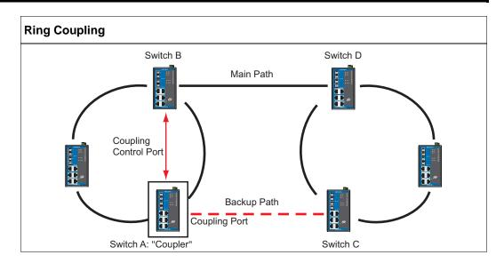
To support the Ring Coupling function, select two EDS-508A/505A (e.g., Switch A and B in the above figure) in the Turbo Ring and another two EDS-508A/505A in the adjacent Turbo Ring (e.g., Switch C and D).
