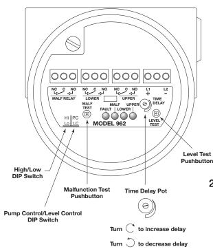
Figure 14 **Model 962 Line Power Configuration**
