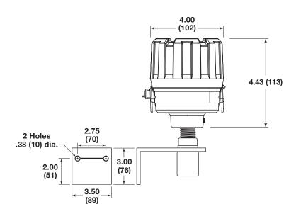
4.00 (102) 3.95 (100) 1.8 (46) Typical Actuation length for NPT connection
