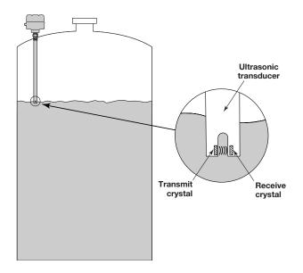
Ultrasonic signal transmission across transducer gap
