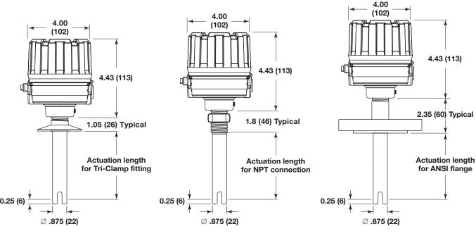
Model 961 with Tri-Clamp® 16 AMP Fitting
