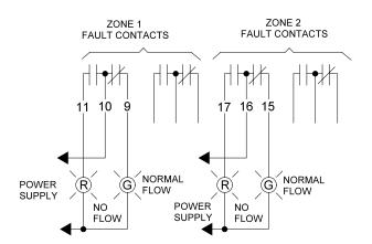
Figure 10. External Flow-No Flow Lights
