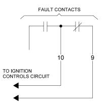
NOTE: DO NOT CONNECT TO HIGH VOLTAGE CONNECT TO CONTROLS ONLY.
