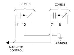
Figure 9. Magneto Grounding
