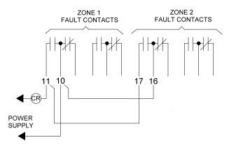
Figure 11. To Energize External Load (relay coil, etc.)
