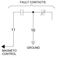
Figure 5. Magneto Grounding
