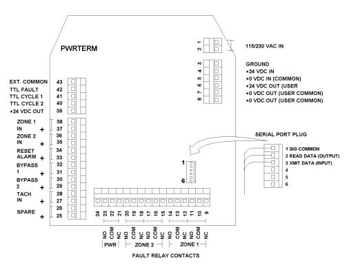
Figure 2. External Connection Terminals
