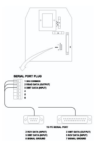
Figure 15. Serial Port Wiring
