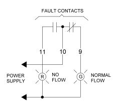
Figure 6. External Flow-No Flow Lights
