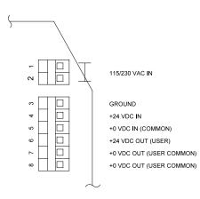
Figure 3. Power Connections
