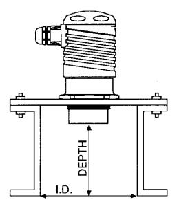
3.1.2 The NEO level transmitter must be installed to avoid interference of the ultrasonic beam cone from the tank side wall. It must be installed such that the beam cone is not interfered by obstructions in the tank such as pipes, nozzles, ladders etc. The transmitter cannot be mounted at an angle (i.e. must be mounted perpendicular to the fluid surface). The NEO will not function in a vacuum.
