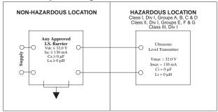
Control drawing for the NEO-50\_1-IS ultrasonic level transmitter approved under the entity concept as an I.S. apparatus
