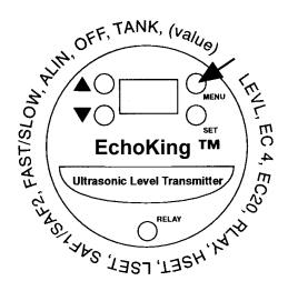
Holding down the "MENU" key will scroll the display through its programming sequence. The display is lit only during the programming mode. It will automatically extinguish when programming is completed and the push-buttons are idle for 30 seconds.
