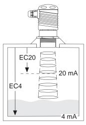
**EC4:** The 4 mA setting for the NEO-50\_1. The EC4 is the distance from the bottom of the NEO-50 1 to the 4 mA set point. This setting is measured in either inches or centimeters on the display. The EC4 setting is typically greater that the EC20 setting.
