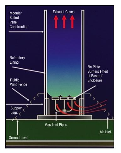
The unique fluidic wind fence that surrounds the KEGF flare ensures an even air flow distribution across the entire burner cross-sectional area.
