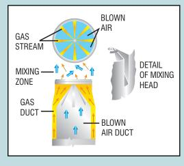
Relief gas moves up the AzDAIR flare's annular duct and is mixed turbulently with air blown up the flare's central duct.
