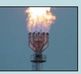
Flare gas exiting the INDAIR flare tip entrains and turbulently mixes 20 times its volume of air as it travels around the tulip-shaped Coanda profile.
