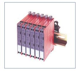
Multiple barriers mounted to 35mm DIN Rail. Each barrier occupies 1/2" of rail space. Once mounted the barrier forms an electrical connection with the rail which now serves as the intrinsic safety ground bus.
