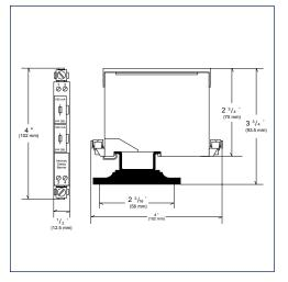
Dimensions of the Series 9000 INTRINSPAK intrinsic safety barrier. All types share a common 1/2" wide housing.
