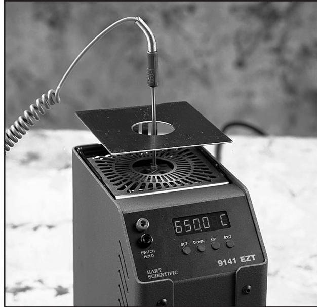
Figure 1 Heat shield installed on 9141calibrator
