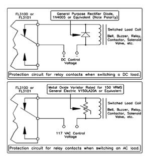
Figure 18: Protection Circuits for Relay Contacts
