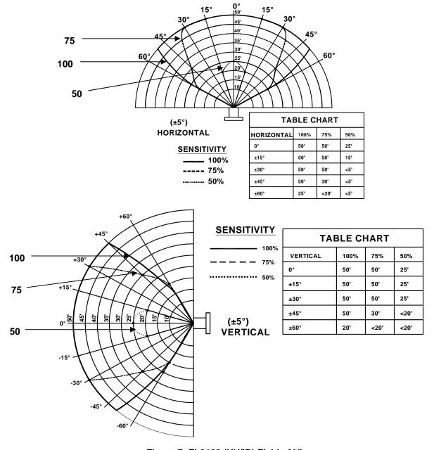
Figure 7: FL3100 (UV/IR) Field of View
