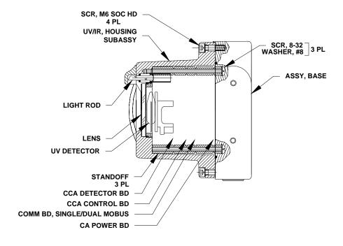
Figure 23: 71100 FL3100 (UV/IR), Final Assembly
