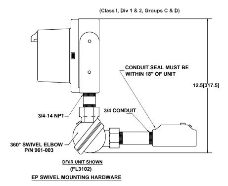
Figure 1: 961-004 Union Swivel Mounting Hardware
