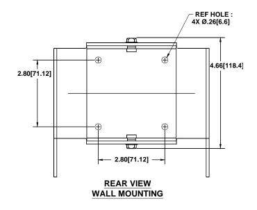
Figure 2: 71172 Rear View Wall Mounting Assembly
