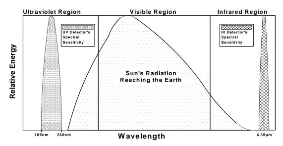
Figure 22: Spectral Response of UV and IR Detectors
