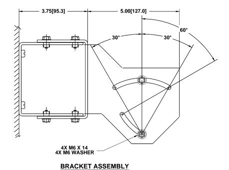
Figure 3: 71172 Rear View Bracket Assembly
