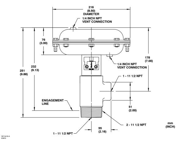
Figure 5. Type D2 Angle Valve Dimensions (Air-to-Open Configuration Shown)
