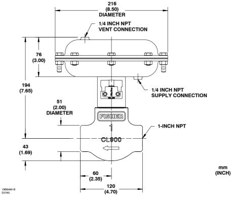
Figure 4. Type D2 Globe Valve Dimensions (Air-to-Open Configuration Shown)
