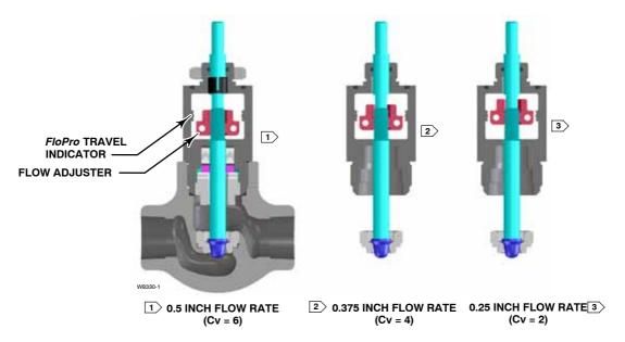
Figure 3. Travel and Flow Coefficients
