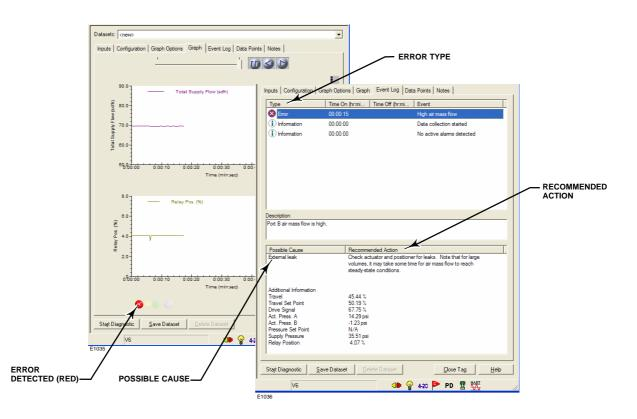
Figure 4. One-Button Sweep—Air Mass Flow Diagnostic
