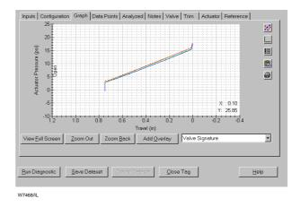
Figure 6. The Valve Signature Display
