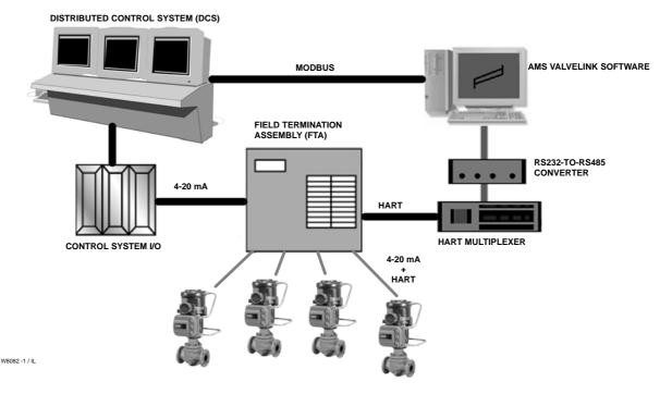
Figure 7. Integrate Information from the Digital Valve Controller into a Non-HART<sup>®</sup> Compatible Control System With AMS<sup>™</sup> ValveLink<sup>®</sup> Software's Modbus Interface
