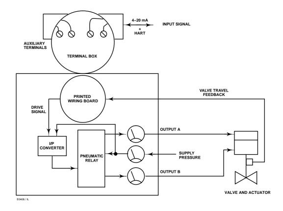
Figure 11. DVC6000 Series Digital Valve Controller Block Diagram
