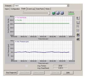
Figure 5. Valve Friction and Deadband Analysis
