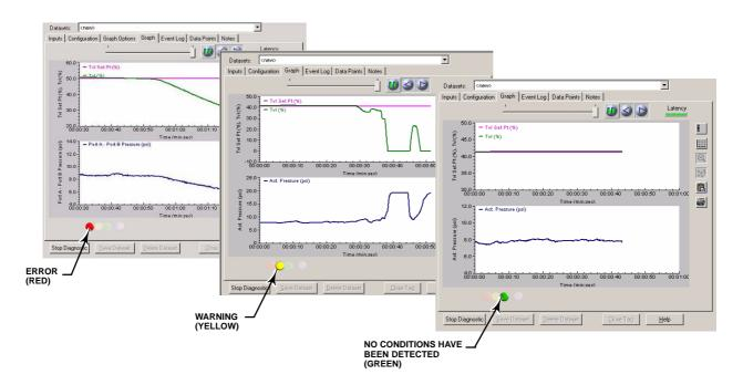
Figure 3. Red/Yellow/Green Condition Indicators, Shown in AMS<sup>™</sup> ValveLink<sup>®</sup> Software
