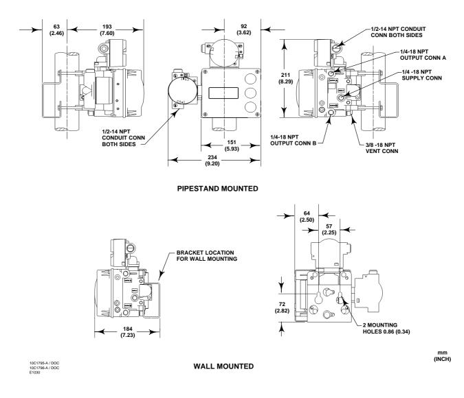
Figure 15. Dimensions for Remote-Mounted Instruments—Type DVC6005 Base Unit
