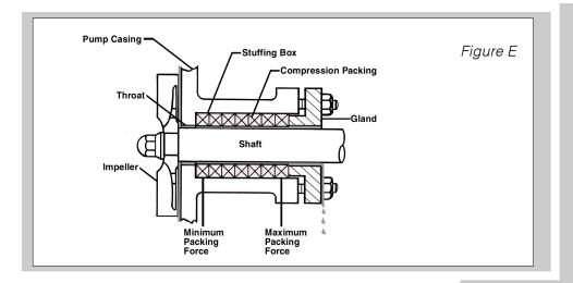
One major group of dynamic seal designs employs the theoretical absence of any rubbing contact between the mating surfaces. A second, more common group involves rubbing contact between the shaft and the seal surface. This group includes the compression packing design mentioned above, as well as endface mechanical seals (commonly referred to as mechanical seals).
