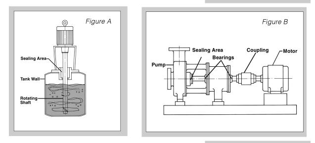
Dynamic seals are frequently located on the shaft of a centrifugal pump. The pump converts the electric motor's rotating energy into velocity, or pressure energy of the liquid or gas being moved.
