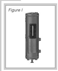
As part of these fluid control systems, many API/ANSI plans require an external tank assembly. Commonly referred to as 'seal pots,' these supply tanks serve as a reservoir of clean, pressurized barrier fluid to double or tandem seal assemblies (fig. I). These tanks, or seal pots, generally utilize either a high-level or low-level liquid switch. In some instances both types are used.
