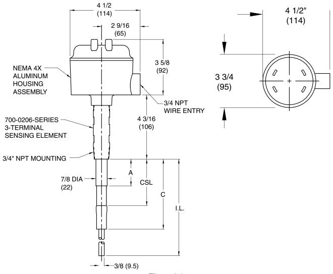
Figure 2-3 Mounting Dimensions, Integral Z-tron III Level Control
