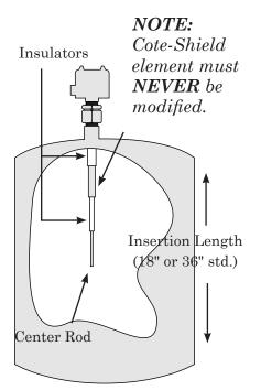
Note: Any changes to probe length after calibration requires re calibration to ensure proper operation.
