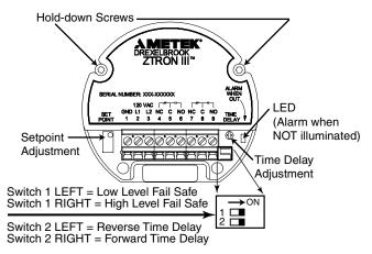
Figure 3-1 Z-tron III Operating Controls and LED
