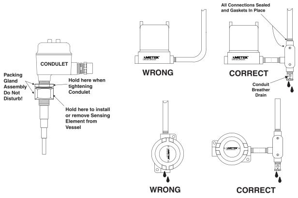
Figure 2-2 Z-tron III Level Control Installation Guidelines
