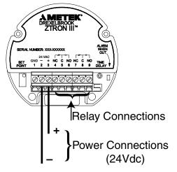
Figure 2-6 Wiring the (24 VDC) Electronic Unit
