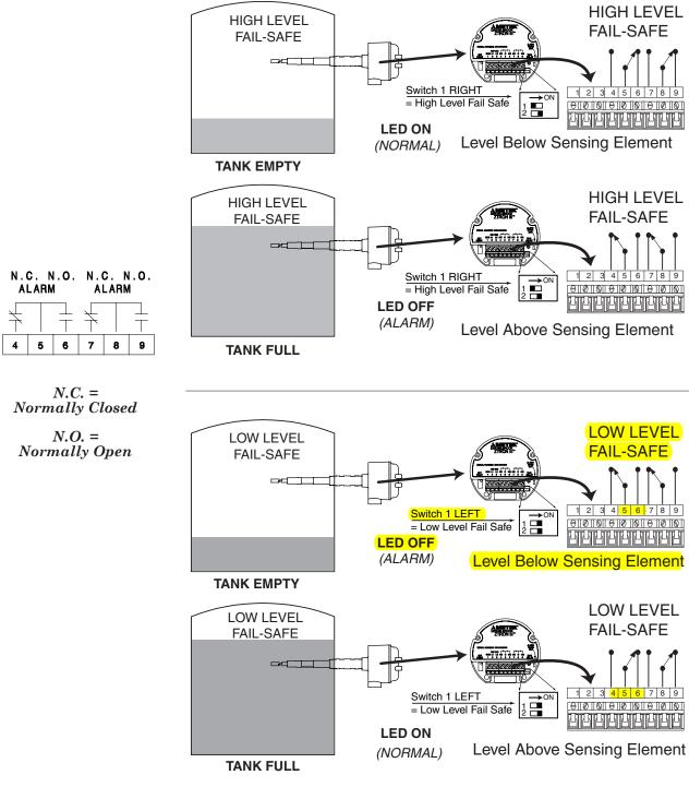
Figure 2-8 Wiring the Relays
