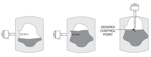
Figure 4-1 Level Below Horizontal Sensing Element Figure 4-2 Level Above Horizontal Sensing Element Figure 4-3 Level Covering Vertical Sensing Element
