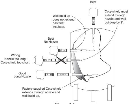
Figure 2-1 Z-tron III Level Control Mounting Recommendations
