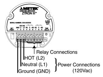
Figure 2-5 Wiring the (120 VAC) Electronic Unit
