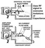
Figure 1-2 RF Admittance Probe with Cote-Shield
