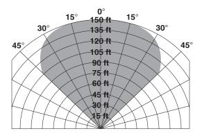
Field of View at Indicated Distance in Feet for **Methanol** at **Very High** Sensitivity (1  $\times$  1 foot)
