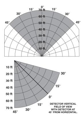
Field of View at Indicated Distance in Feet for **Isopropanol** at **Very High** Sensitivity (6 in. x 6 in.)
