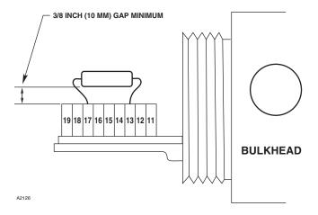
Figure 6—EOL Resistor Installation
