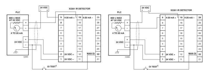
Figure 11—X3301 Detector Wired for Isolated 4 to 20 mA Current Output (Sourcing)
