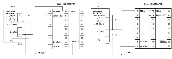
Figure 9—X3301 Detector Wired for Non-Isolated 4 to 20 mA Current Output (Sourcing)
