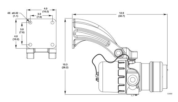
Figure 3—Q9033B Mounting Bracket Dimensions in Inches (cm) (See Figure 1 for Correct Detector Orientation.)
