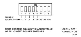
Figure 16—Address Switches for X3301
