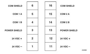
Figure 13—Wiring Terminal Identification for X3301 EQP Model
