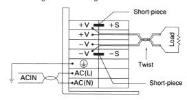
(2)When using remote sensing function
