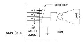
(2)When using remote sensing function
