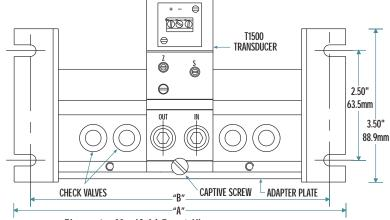
Figure 1 - Manifold Front View
