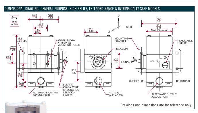
The Type 1000 has long been a standard in the I/P & E/P industry. With a built-in booster, the T-1000 provides a flow capacity up to 12 SCFM, making it a versatile transducer for many applications.
