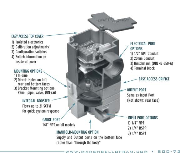
The secret to the Type 2000's precise, reliable performance under a variety of demanding environmental conditions is a patented piezo-ceramic actuator with many industry-wide firsts.
