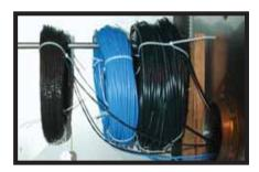
The cables were tested, as suspended, in a high temp oven.
