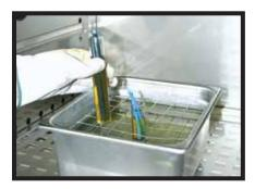
The oil bath test, conducted as specified in UL 1277.
