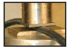
The DataTuff cable fails only after a ton of crush pressure.
