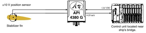
The **API 4380 G** switches are set to Input select "V", Output select "I" and A=5, B=7, and C=6 for ±10 V input and 4-20 mA output. The **API 4380 G** powers the output loop, thus eliminating the need for an additional power supply. The 2000 V<sub>RMS</sub> 3-way isolation of the module protects against unexpected ground loops and electrical noise.
