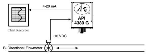
The API 4380 G is set up for a ±10 V signal and 4-20 mA output. The module switches are set to Input = "V", ABC = 576 and Output = "I"
