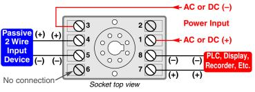
Using the built-in 18 VDC loop supply to power a passive input device
