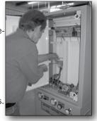
mination ferrules and wire tags on every wire, well-routed tubing, separated low and high voltage wiring, and high quality enclosures and finishes. It also means rigorously testing every electrical or process tubing point in the panel with either high pressure air or hydraulics, calibrating all transducers to the instrument, and checking every function in the panel.
