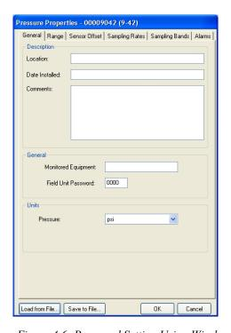
Figure 4.6: Password Setting Using Wireless Instrumentation Manager
