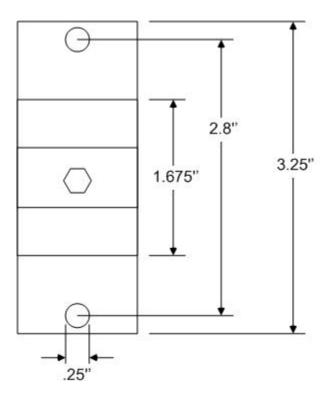
Mounting bracket dimensioned drawing
