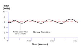
Figure 6.12: Condition "Chatter" Elimination Due to Time Deadband
