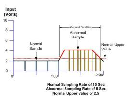
*Figure 6.7: Example of Abnormal Sampling Rate Setting*
