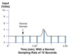
Figure 6.3: Correct Sampling Rate
