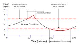
*Figure 6.9: Normal Upper and Lower Value Example*
