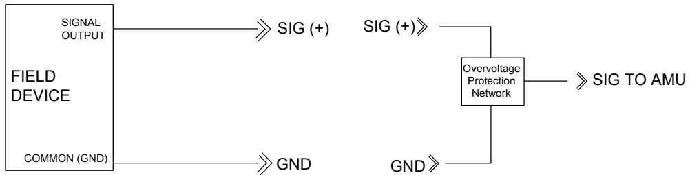
TYPICAL 2 WIRE 4--20mA FIELD DEVICE WIRING
