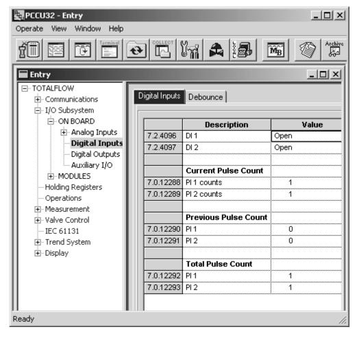
Figure 2–3 Totalflow PCCU32 I/O Subsystem\ON BOARD\Digital Input
